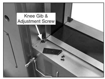
Figure 64. Knee gib and adjustment screw.
